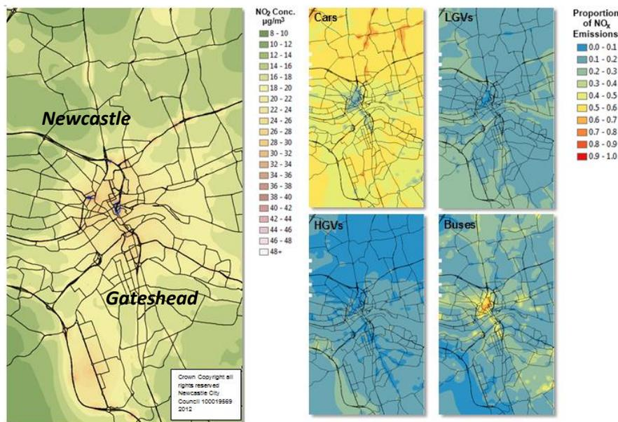
**Figure 3.** Concentrations of NO<sub>2</sub> and source apportionment of NO<sub>x</sub> in the 2021 'do-minimum' case
