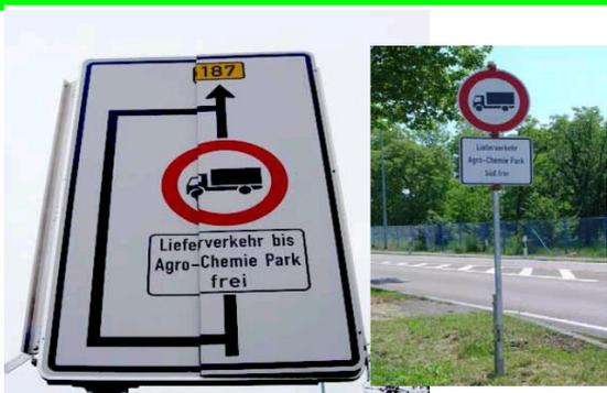
Traffic signs for HDV Deviation, which are opened manually
