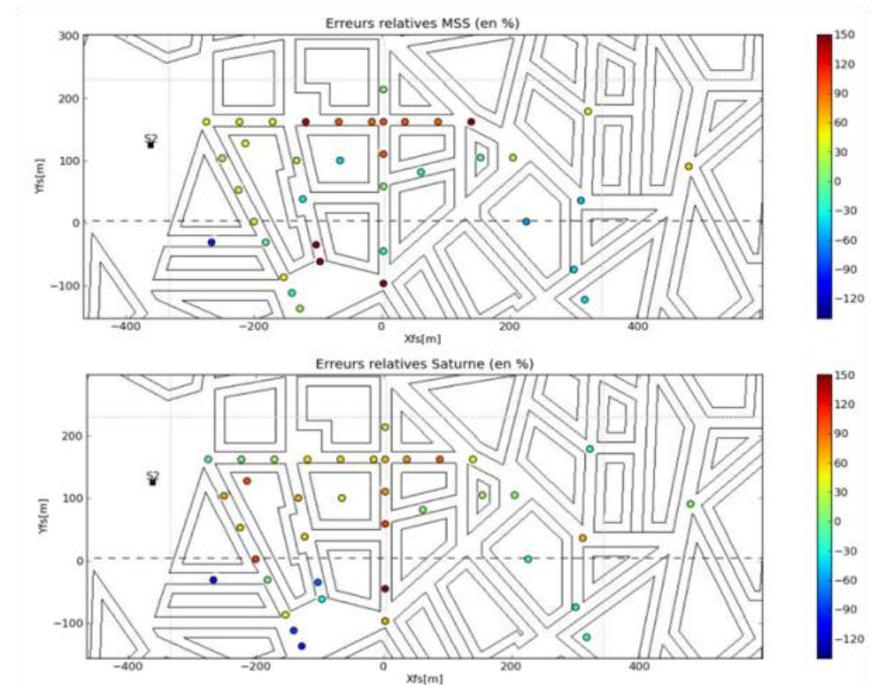
*Concentration field at a height of 7.5 m and relative errors compared to observations for continuous release from source S2 (PMSS at the top and SATURNE at the bottom)*
