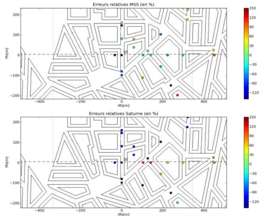
*Concentration field at a height of 7.5 m and relative errors compared to observations for continuous release from source S5 (PMSS at the top and SATURNE at the bottom)*
