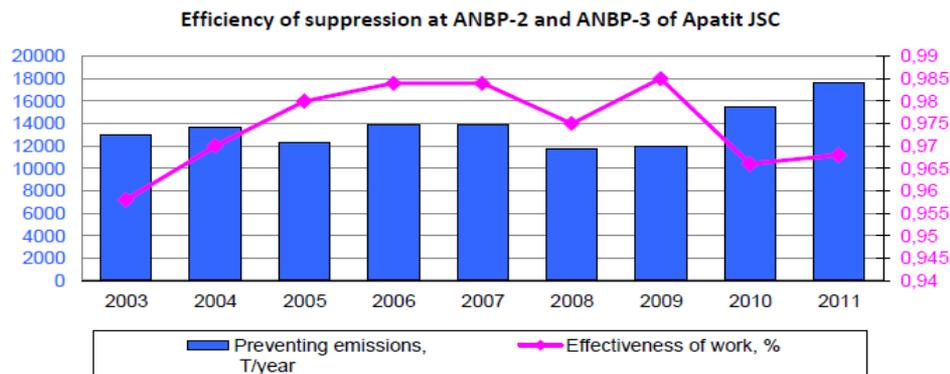
Figure M3.2. Efficiency of dust suppression at ANBP-2 and ANBP-3
