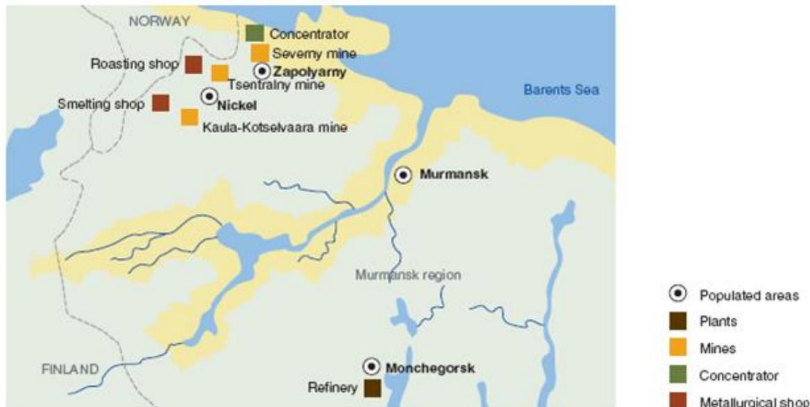
The extracted ore is processed at the Concentrator, producing collective copper and nickel concentrate. The Concentrator produces copper and nickel concentrate that is further transferred to the Roasting section of the Smelting shop for further processing.
