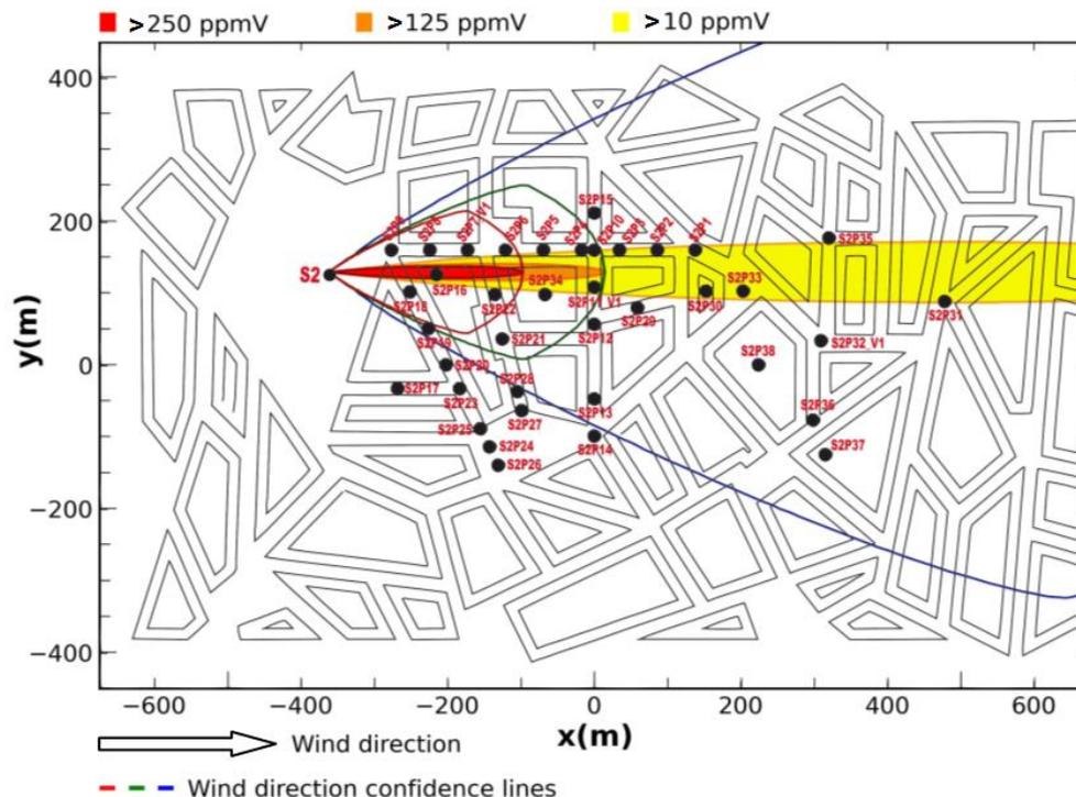
Horizontal distribution of average near ground concentrations for a continuous release from source S2 simulated with a models of type I (model 101)
