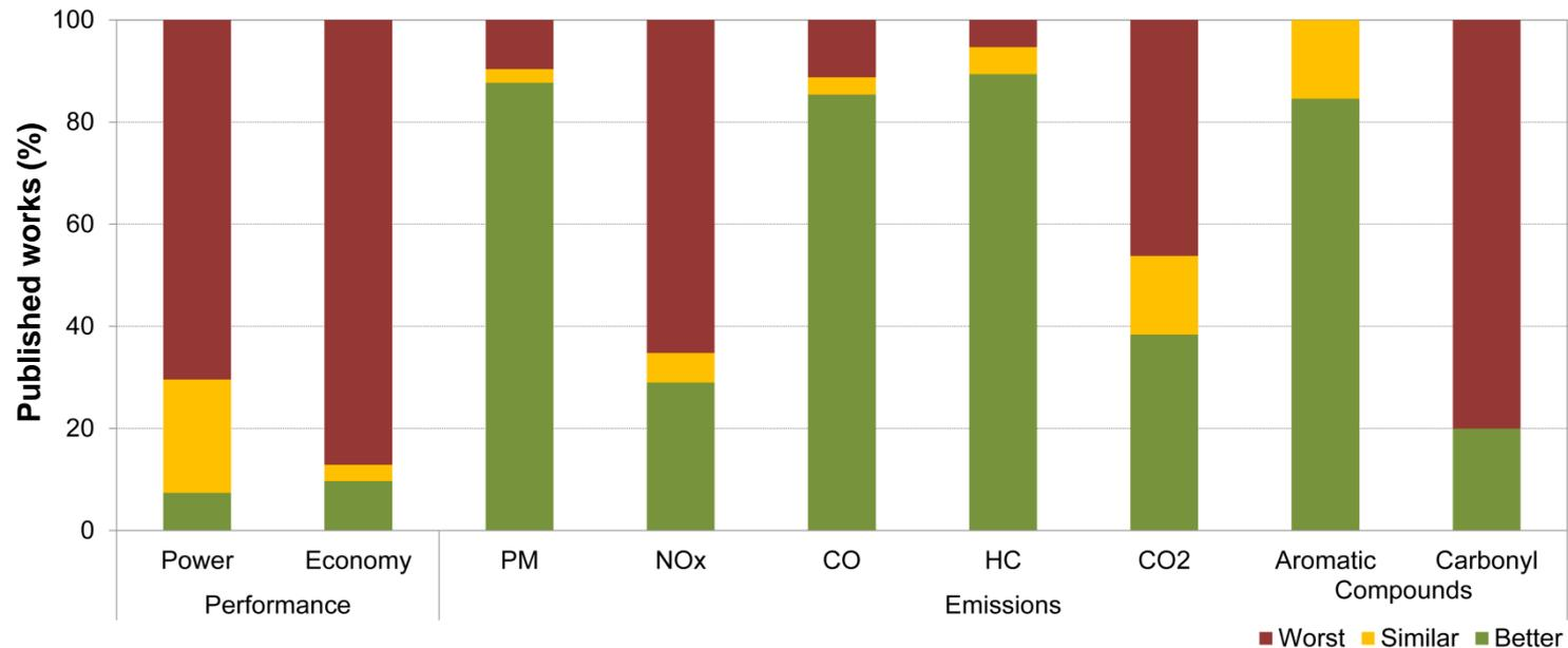
**B20 with higher combustion efficiency and lower emissions than diesel and other blends**
