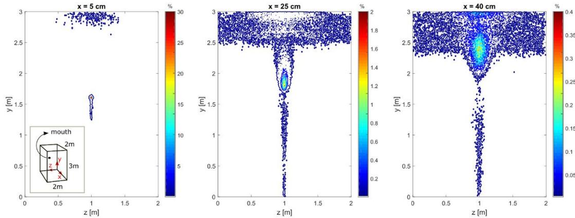
**Figure 3.** Droplet number concentration fields on transversal sections at 5, 25 and 40 cm from the mouth
