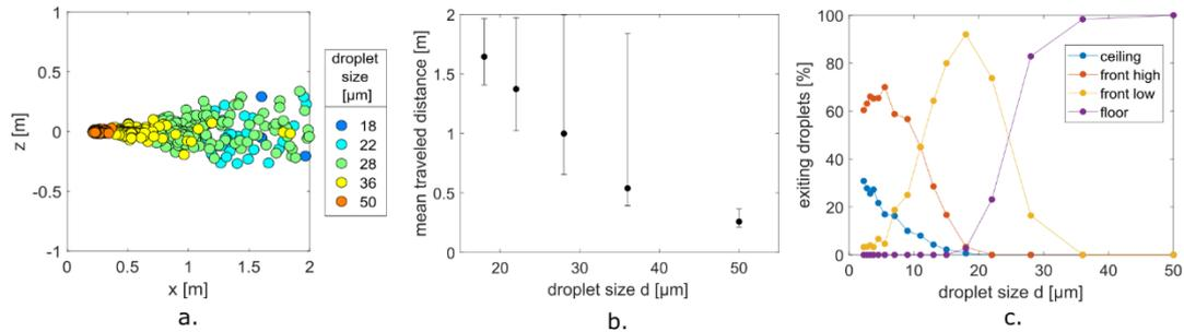
**Figure 2.** a. Settled droplets; each circle corresponds to a droplet, circle color is related to droplet size, b. mean, maximum and minimum traveled distances before settling and c. percentage of particles of each size class exiting through different domain zones
