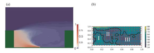
Figure 2. (a) Simulated normalised concentration field (C/Cmax) and (b) scatterplot of the Cleaning Effect values, the thick black line designates the 50%
