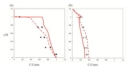
Figure 1. Simulated normalised concentration profiles at the (a) upwind and (b) downwind building walls for a street canyon with AR = 1. Current LES is presented by the continuous red line, the LES by Li et al. (2008) by the dashed line. the wind tunnel data by Pavageau (1996) are presented with squares and by Meroney et al. (1996) with circles. z/H is the non-dimensional height, where H is the building height.
