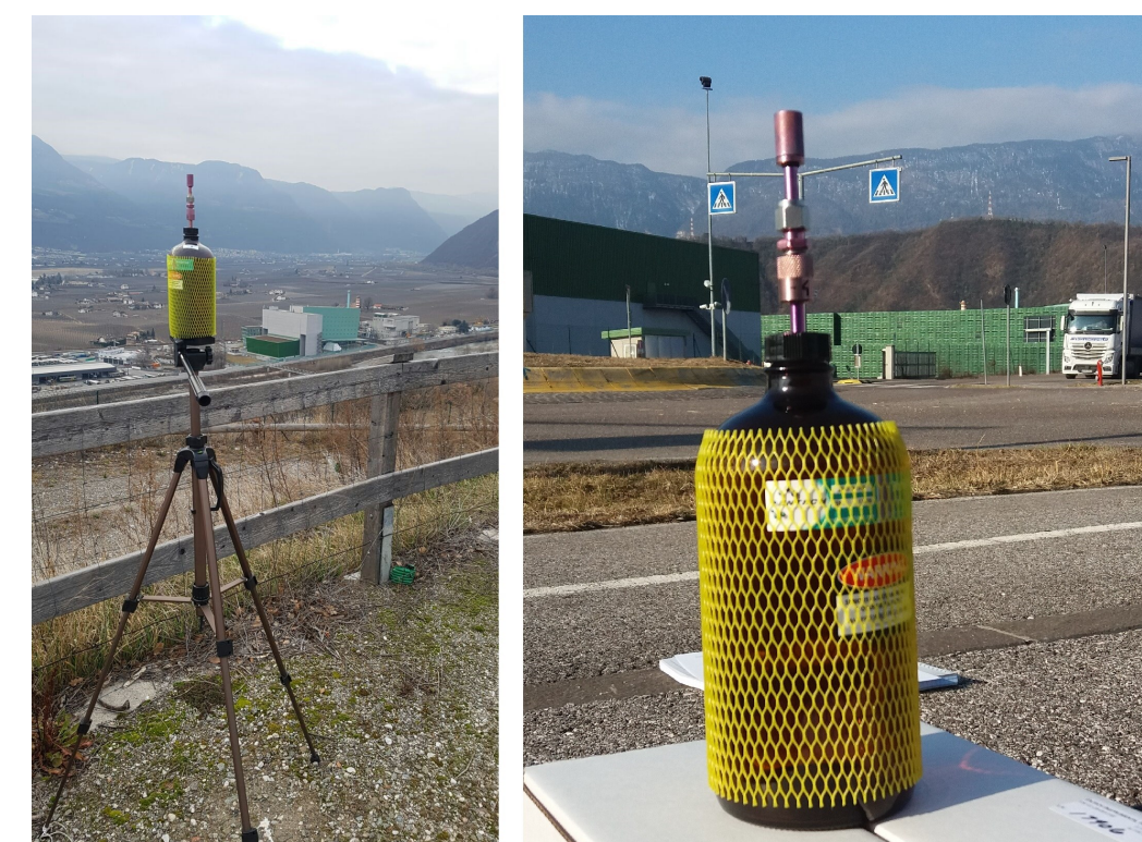
Figure 3: Vacuum bottles used for the sampling of ambient air during BTEX
