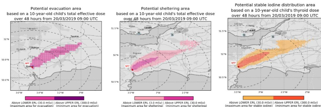
**Figure 3.** Potential areas for protective actions for health: evacuation area, sheltering area and distribution area for stable iodine. Two emergency reference levels (ERLs) are applied to the total effective dose for evacuation and sheltering, and two ERLs are applied to the thyroid dose for the stable iodine; these are shown below each graphic.
