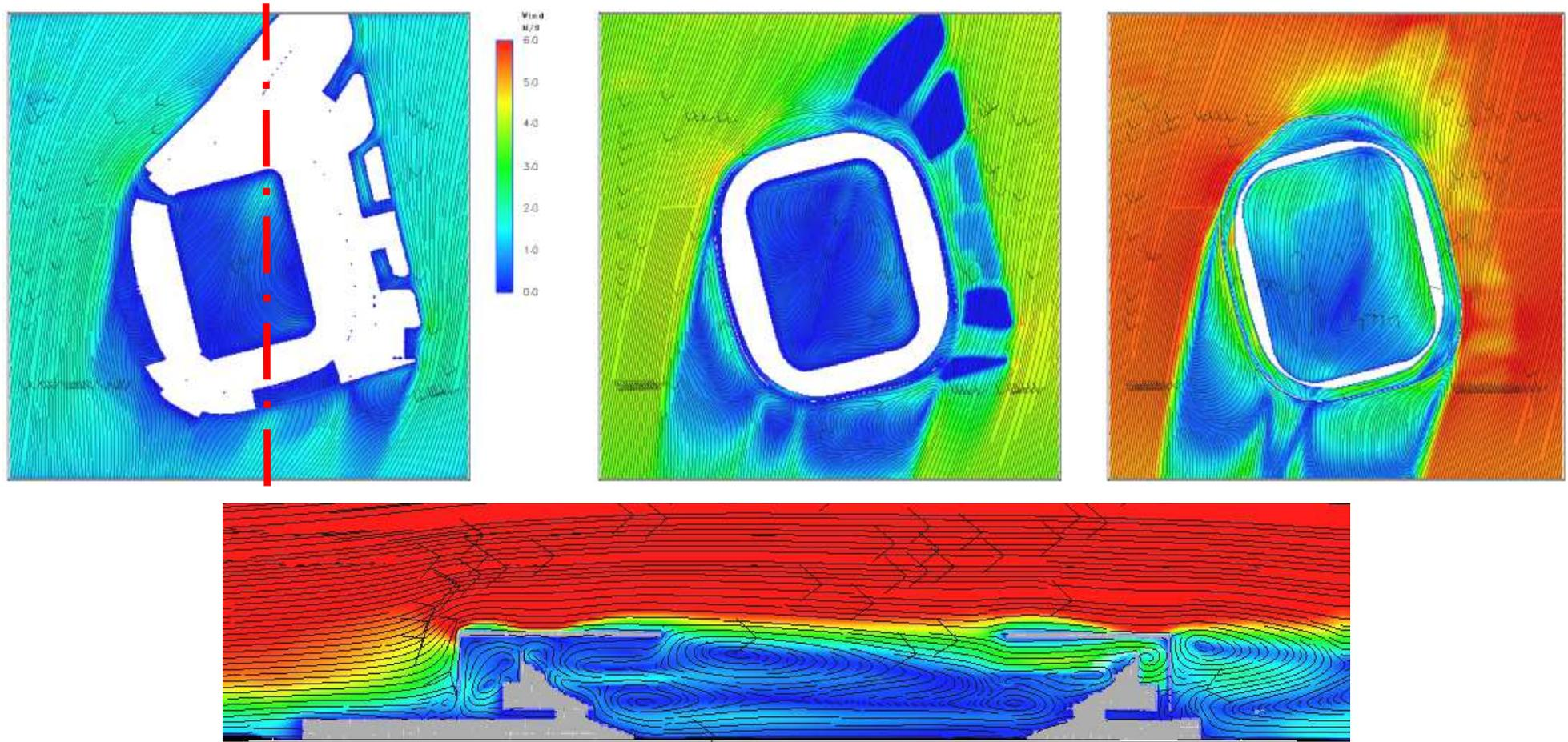
Horizontal and vertical cuts of the flow field in PMSS domain **N03** at 0830 Z. The horizontal cuts are presented at 4 m (middle of the lower rostrum), 13 m (middle of the intermediate stands) and 21 m (middle of the upper stands).
