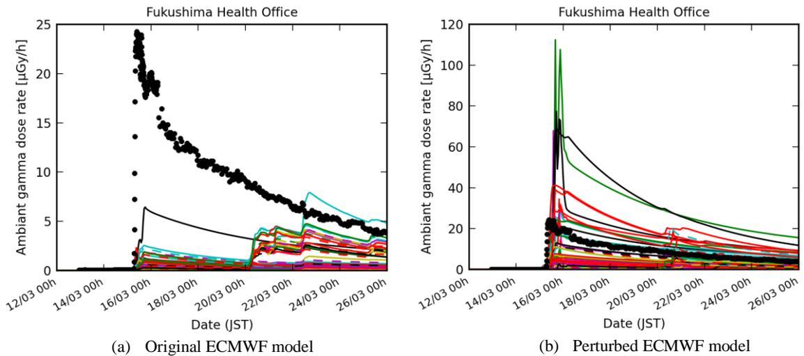
**Figure 5.** Gamma dose rate of each outputs of the meteorological ensemble compared to the observation for the Fukushima Health Office station.
