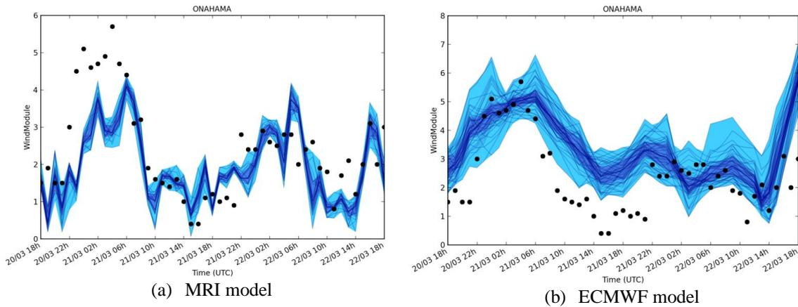
**Figure 1.** Wind module ( $\text{m}\cdot\text{s}^{-1}$ ) of the meteorological ensembles (in blue) compared to the AMeDAS observations (in black) for the Onahama station.
