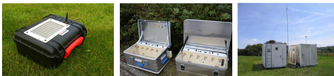
Figure 2. Beta counting proportional counter (Berthold-LB123) (left), air sampler VEGA (middle), and 6-m sonic anemometer for wind measurement (right).
