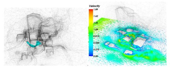
(a) Tracer Iso-surface (b) Complex turbulent air flows at ground-level **Figure 5** Three-dimensional view of Adaptive mesh-refinement around the "Walkie-Talkie" building area, Central London together with: (a) a tracer isosurface and (b) the complex flow field near ground level.
