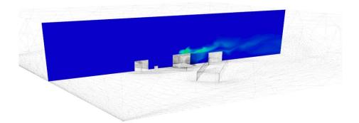
Figure 2 Vertical Cross-section through centre of computational domain for the dispersion of Tracer 4, with source at top of building.
