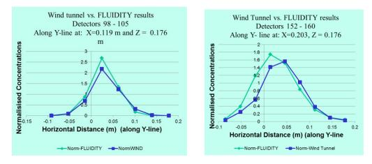
Figure 4 Comparison of simulated normalised FLUIDITY tracer concentrations with wind tunnel measurements from the Enflo wind tunnel.
