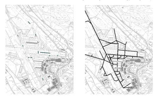
Fig. 3; Monitor versus scenario calculation (Zürich Airport). Left: Snap-shot of aircraft traffic in a monitor calculation, showing the line segments that 12 aircraft pass in the depicted 10-second interval. Right: Stationary line sources for taxiway emissions in a scenario calculation.
