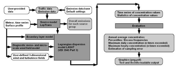
Fig. 1; General structure of the program system LASPORT.
