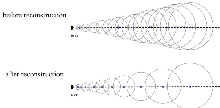
Figure 1: Puff dispersion model before and after plume reconstruction algorithm.
