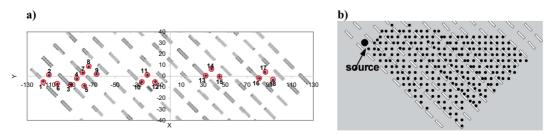
Figure 1. Measurement positions for the -45 degree case. a) towers for velocities, b) concentrations. Wind blows from the left.
