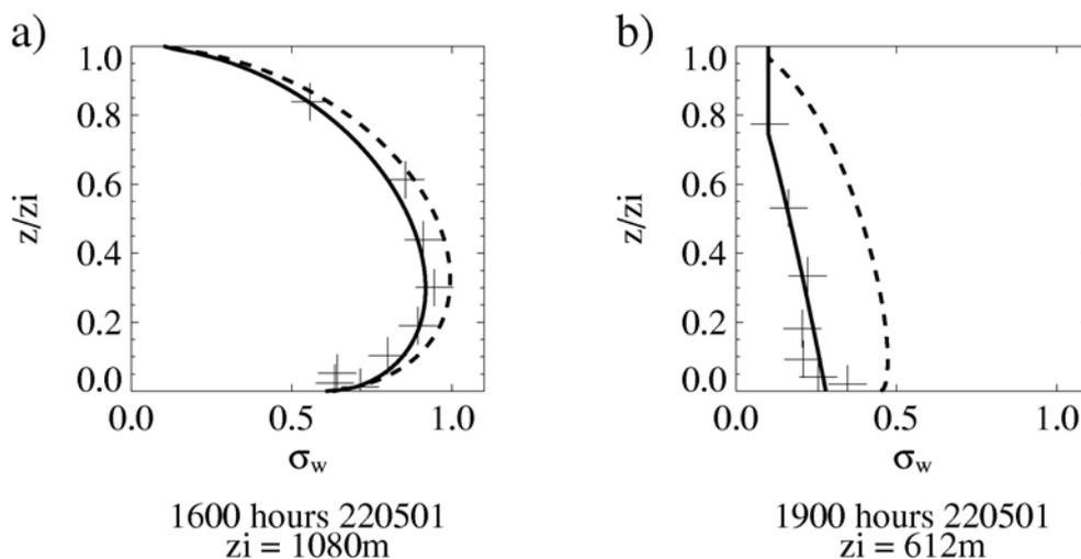
Figure 1. Observed  $\sigma_w$  (crosses), predicted  $\sigma_w$  using UM mesoscale meteorological data (dashed lines) and predicted  $\sigma_w$  using observed meteorology (solid lines) at Cardington in (a) unstable conditions and (b) neutral/stable conditions.
