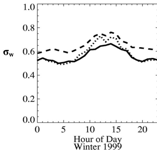
Figure 2. Mean diurnal cycles of 15m observations of  $\sigma_w$  (solid lines), predicted  $\sigma_w$  using UM mesoscale meteorological data (dashed lines) and predicted  $\sigma_w$  using observed  $u_*$  in UM defined stable conditions (dotted lines) for the winter 1999 measurement campaign in Birmingham.
