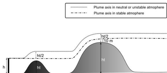
Fig. 21: Modelling of relief influence in the atmospheric dispersion
