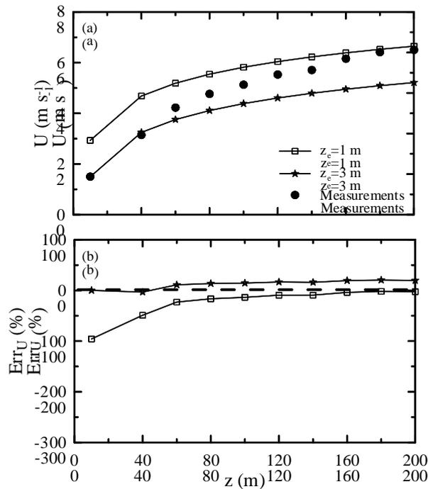
Figure 3. Vertical profiles of (a) wind speed and (b) error when the angle of rotation of the wind vector is less than 22.5° in the height range between 10 and 200 m a.g.l (neutral atmosphere).
