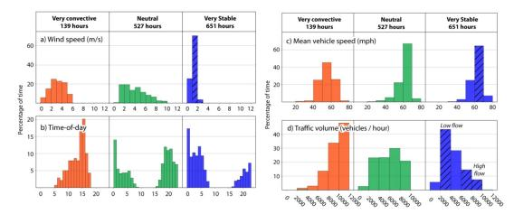
Figure 2. Characteristics of selected data as used in conditional analysis of roadway dispersion: data are summarised by stability groups for: a) wind speed ( $ms^{-1}$ ) b) time-of day c) vehicle speed (mph) & d) traffic volume (vehicles/hour). All data were used for downwind decay analysis, and hatched data under 'very stable' group were used for wake effect analysis.
