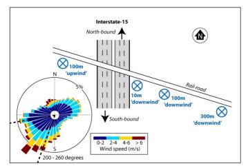
Figure 1. Monitoring positions and wind rose for the Las Vegas roadway study, showing wind sector 200-260 degrees (dashed) as used for conditional analysis.
