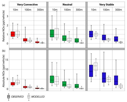
Figure 3. Declines of observed and modelled concentrations with distance from roadway for selected stability groups: (a) shows concentrations relative to 10m median value, which is set to unity; (b) shows absolute concentrations.
