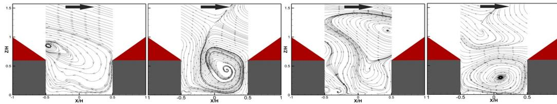
Figure 2. The four most dominant spatial modes (topos) displayed with pseudo-streamlines for pitched roof geometry: from the left: a) first mode, b) second mode, c) third mode, d) fourth mode. Black arrow on the top shows the direction of the approaching flow.
