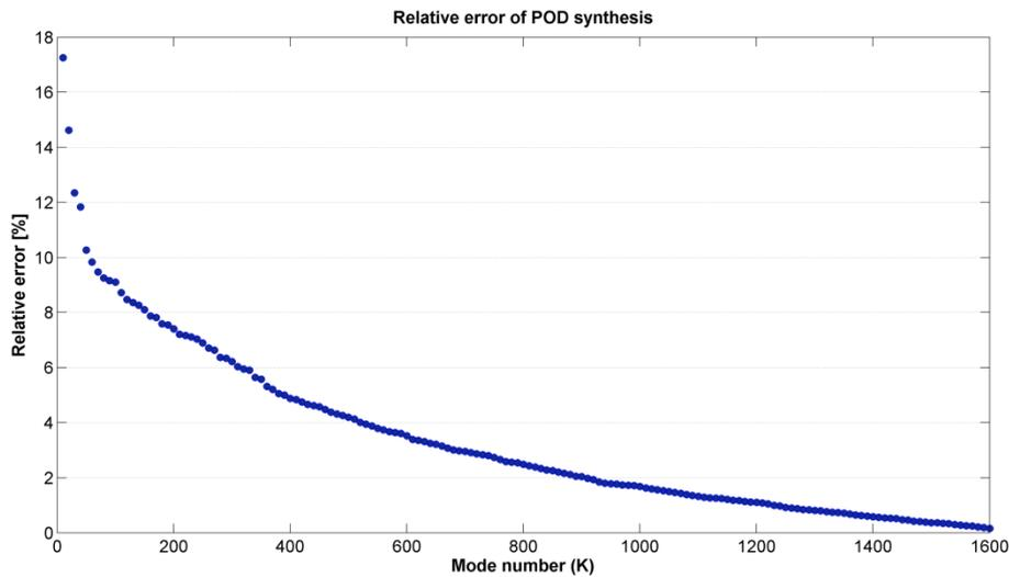
Figure 5. Relative error of synthesis for pitched case. The error is calculated for 1600 snapshots with all 1600 modes and averaged over all snapshots. Calculation is based in Frobenius norm.
