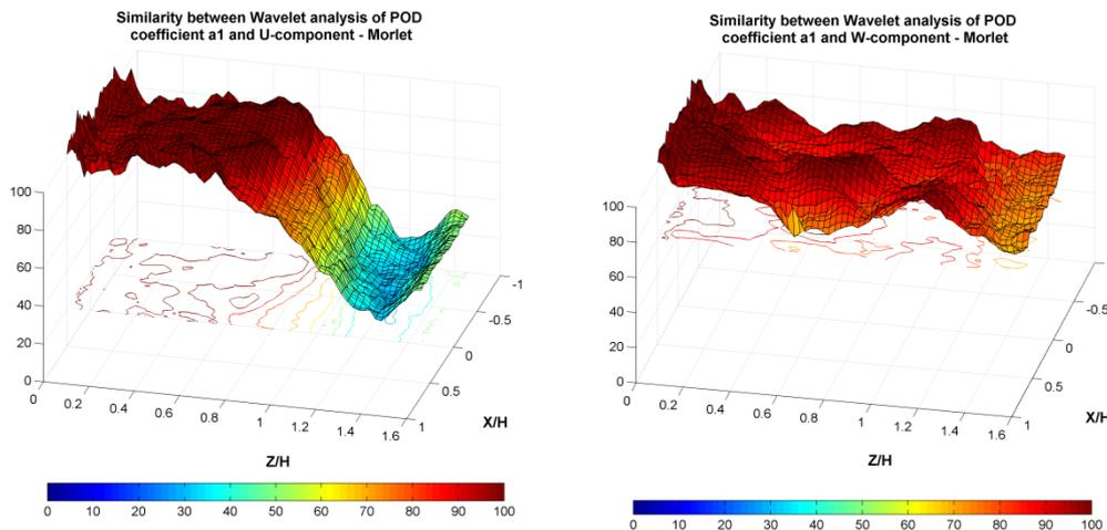
Figure 8. Similarity between wavelet scalogram of POD coefficient  $a_1$  (whole spatial extent of the street canyon) and U-component (left) or W-component (right) at various positions.
