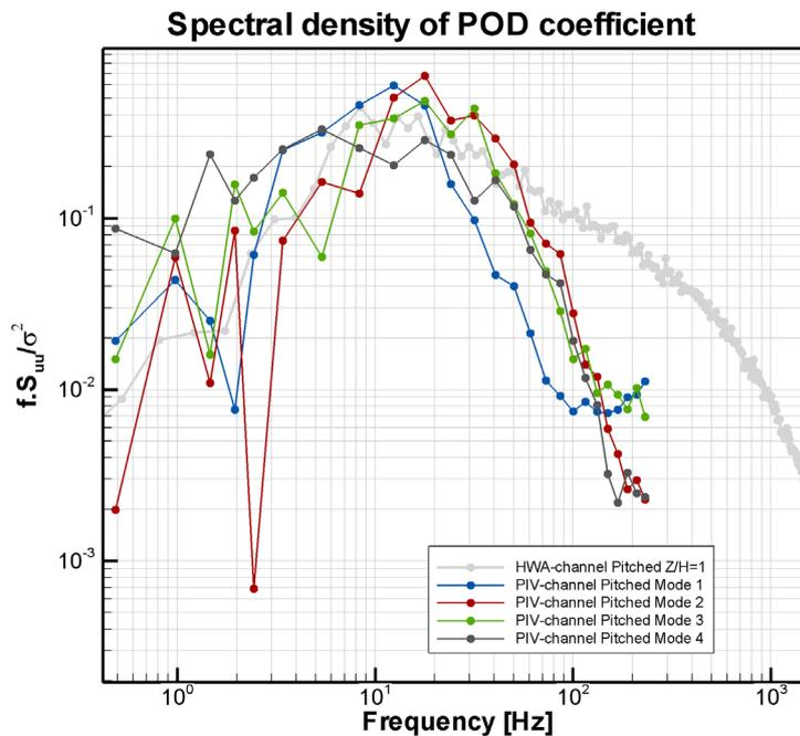
Figure 7. Fourier spectral analysis of U-component of velocity at Z/H=1 (obtained from HWA) - light grey line. The spectral analysis of POD expansion coefficients (obtained from PIV) - other colours.
