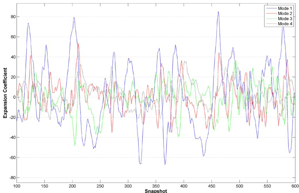
Figure 3. Example of temporal evolution of expansion coefficients for four POD modes. Each colour corresponds to one POD mode.
