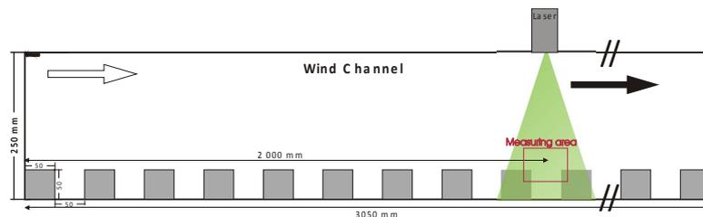
Figure 1: Scheme of the channel and laser sheet. Investigated XZ plane is in the middle of channel.
