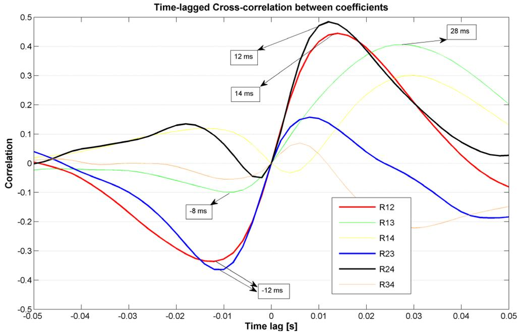
Figure 4. Time-lagged cross-correlation between particular expansion coefficients (e.g. R12=correlation between expansion coefficients of Mode 1 and Mode 2). Thick line labels the correlations with significant maximum.
