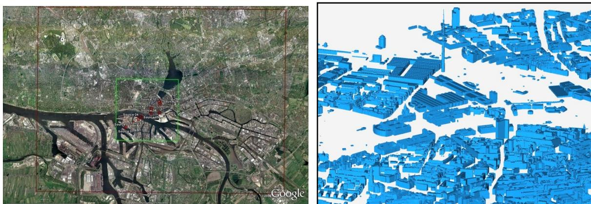
Fig. 1: (a) Top view on the 16km x 12km and 4km x 4 km domains. Lake Alster, River Elbe and the city centre are landmarks which provide orientation. (b) Sample of the 3D high-resolution geometry. The Hamburg Fair ground, the TV tower and parts of Hamburg University are easily identifiable.
