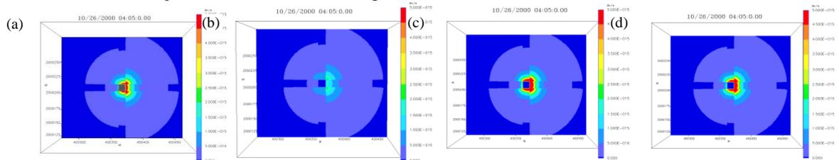
Figure 3. Gamma dose rates in planes at 0 m (a), 10 m (b), 11 m (c) and 20 m (d) AGL due to  $^{60}\text{Co}$  particles deposited on the cube walls.
