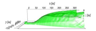
The 2000 ppm 3D contour plot gives an idea of the shape of the contaminant cloud. Up to 50 m from the source the dynamic of the plume is dominated by the initial momentum while at farthest distances it is regulated by buoyancy. From 150 m to 300 m a lowering of the contour at the centre can be noticed, the dense cloud weight induces gravity spreading and radial outflow velocity increasing the contaminant concentration on the sides of the plume.
