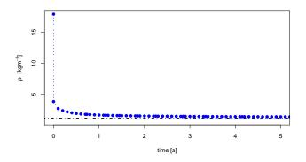
In the very first instants of the simulation the density gradient is very steep and the initial density is very quickly lost, the loss is due to the fast vaporization of the liquids in the aerosols.
