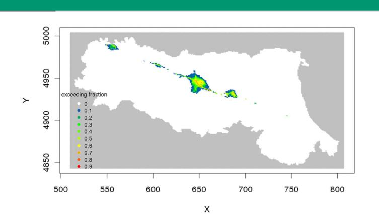
Figure 7: Fraction of land where  $NO_2$  annual mean exceeded the  $40\mu g \cdot m^{-3}$  threshold, as estimated by the UltraPESCO module.
