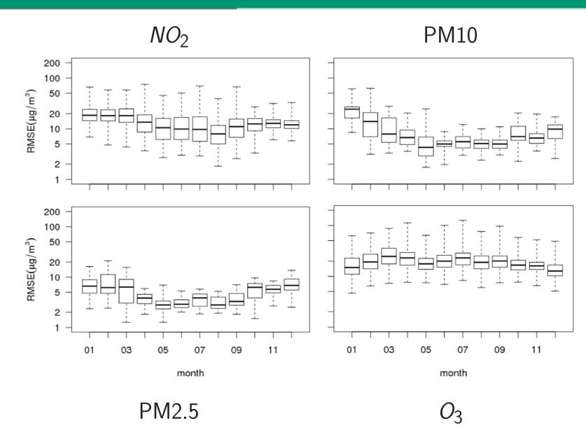
Figure 4: Cross-validation of the geostatistical module PESCO: monthly minimum, maximum, median,  $25^{th}$  and  $75^{th}$  percentile of the root mean square error, represented as box-and-whyskers plots
