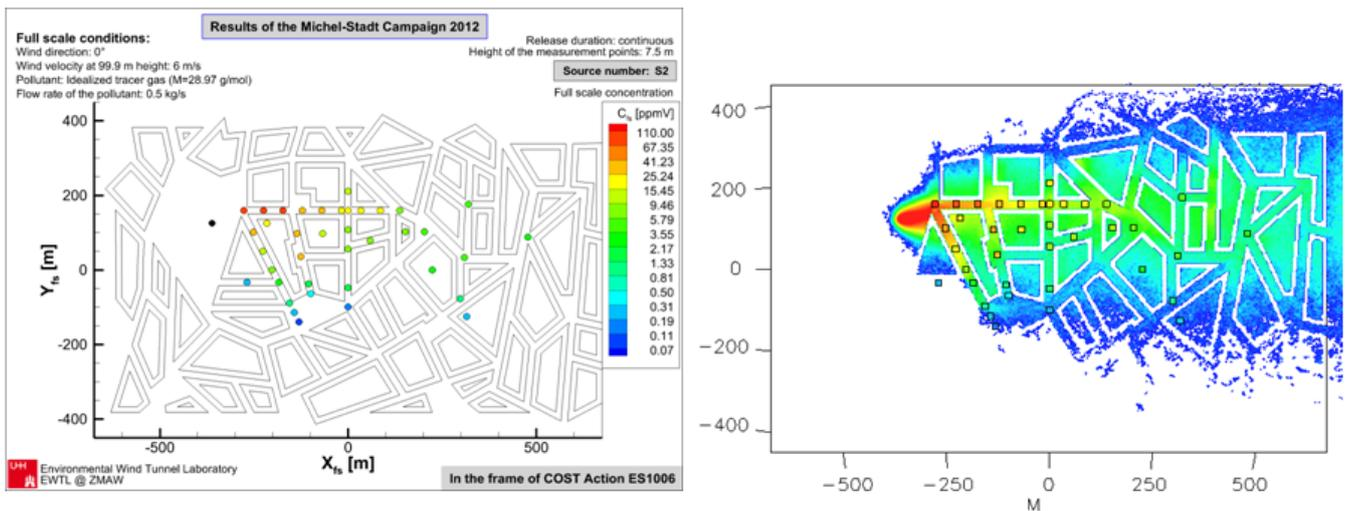
Figure 2. Sketch of the Michelstadt geometry and S2-case measurements (left) and example of the concentration fields from a Lagrangian particle dispersion model run (right)
