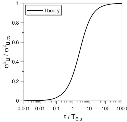
**Figure 1:** Dependence of  $\sigma_u$  on the sampling duration  $\tau$ .
