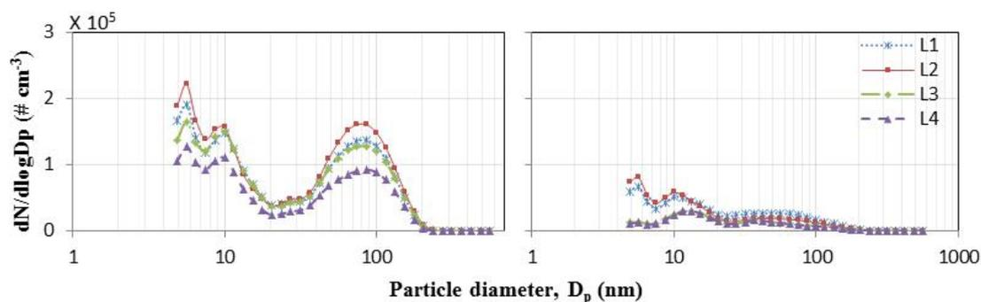
Figure 2: Particle size distribution at various sampling points on (a) 7 August 2012 (weekday) (b) 11 August 2012 (weekend).
