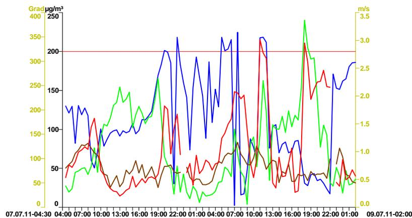
Figure 3. Observed NO<sub>2</sub> concentrations (red curve) near the Plabutsch tunnel (south portal) and at a curb site in Graz (brown curve); wind speed (green curve) and -direction (blue curve)
