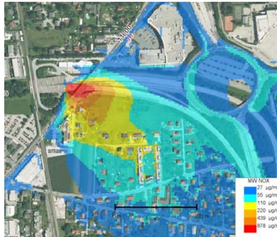
Figure 5. Modelled average  $\text{NO}_x$  concentrations in the vicinity of the southern portal of the Plabutsch tunnel (Scenario 2)
