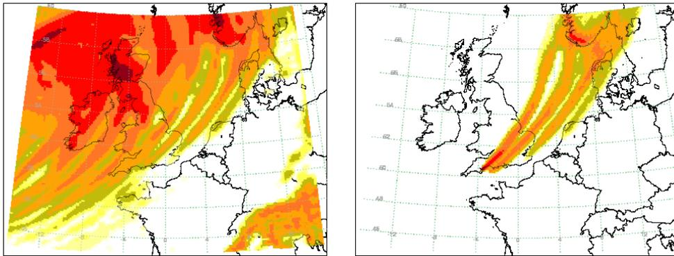
Figure 1. Example 24-hour accumulated precipitation (left) and corresponding NAME predicted wet deposition (right) obtained using 3-hourly instantaneous precipitation fields from the global version of the Unified Model.
