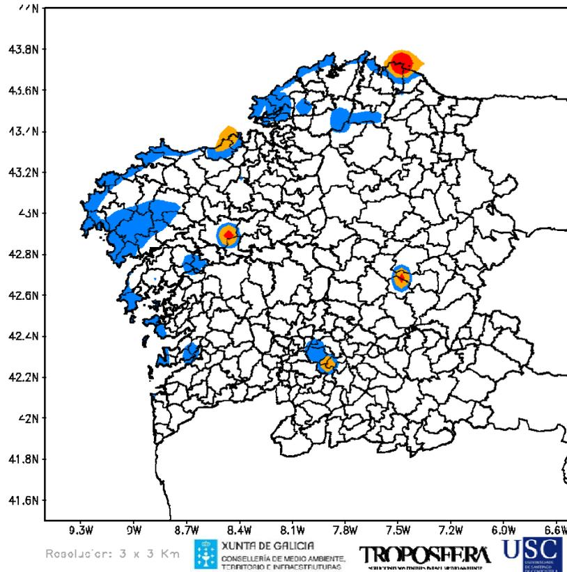
Figure 2. Optimal air quality network design: Areas with exceedances in the upper (orange) and lower (blue) legal air quality thresholds, for any primary pollutant. Red colour shows the threshold value exceedances.
