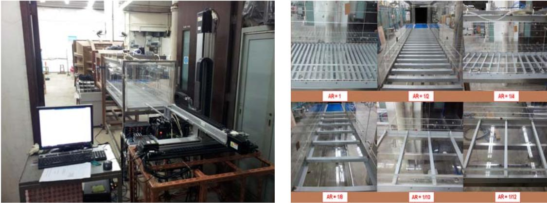
Figure 1. Experimental setup and idealized urban-like models.
