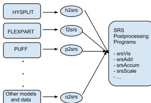
Figure 1. SRS-based postprocessing system
