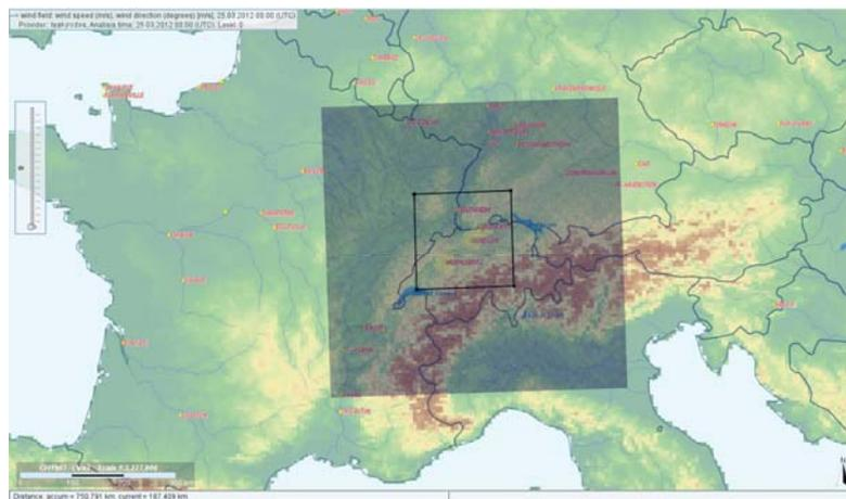
Figure 1. Snapshot of the JRODOS system showing the orography of Switzerland and of the surrounding states. The inner square shows the area currently covered by the data of NWP at ENSI. With the replacement of ADPIC the covered area will be extended to the larger grey shaded square.
