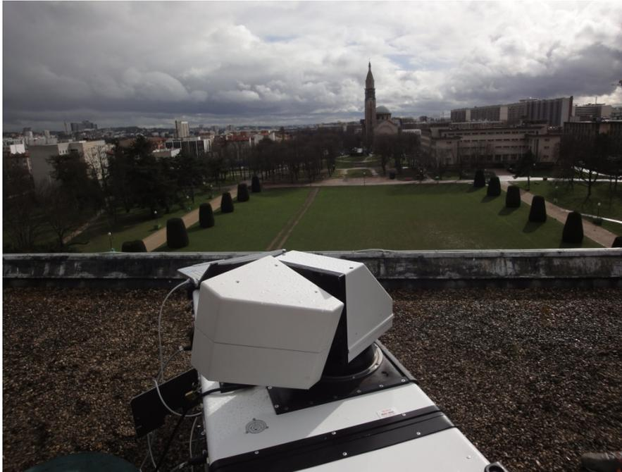
**3D scanning wind LIDAR**
