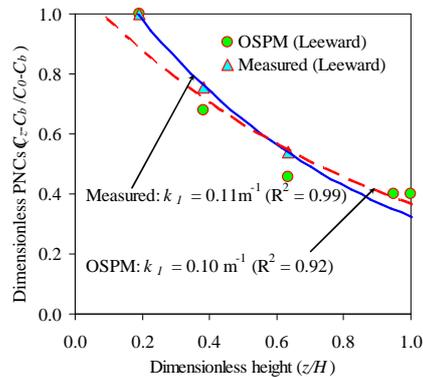
Figure 5. Estimation of exponential decay coefficient ( $k_1$ ) using measured and OSPM modelled data.
