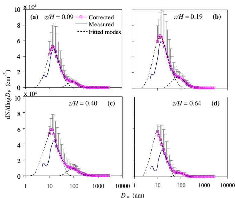
Figure 2. Hourly averaged measured particle number distributions at (a) 1.0, (b) 2.25, (c) 4.62, and (d) 7.37 m of an 11.6 m deep canyon. Distributions have been corrected for particle losses in the sampling tubes of different lengths (Kumar *et al.* 2008d).
