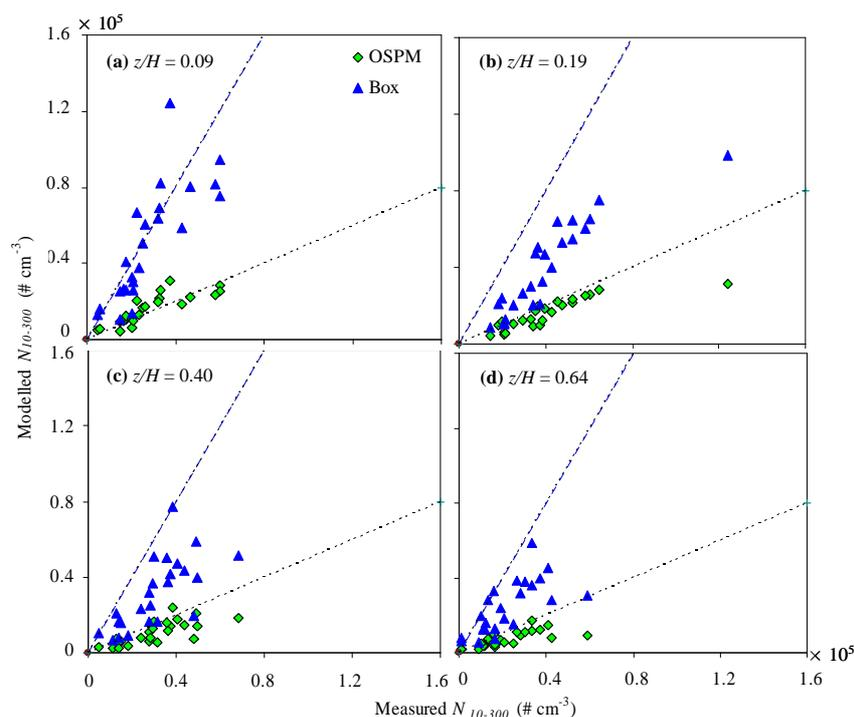
Figure 3. Comparison of hourly averaged measured and modelled nanoparticle number concentrations at the leeward side of the canyon at (a) 1.0, (b) 2.25, (c) 4.62, and (d) 7.37 m heights. Dotted lines cover the range of predictions within a factor of 2 (FAC2).
