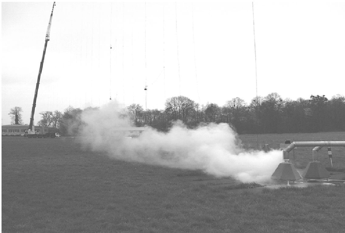
Figure 1. View of a part of the experimental arrangement showing the spill point and vertical steel ropes
