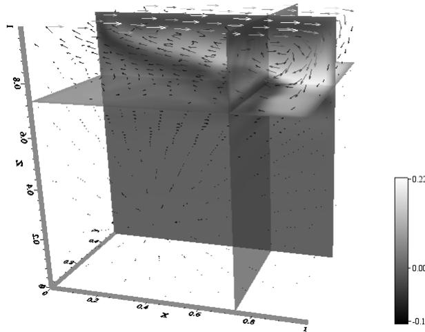
Figure 3. Field of potential temperature, arrows of flow field cross-section through the 3D simulation (planes  $x=0.75, y=0.5, z=0.75$ ),  $Re = 400, Fr = 0.1$
