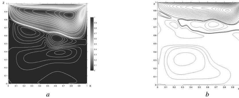
Figure 2. Streamlines of the flow field for  $Fr = 0.1$ : a) 2D, velocity magnitude,  $Re = 100$
