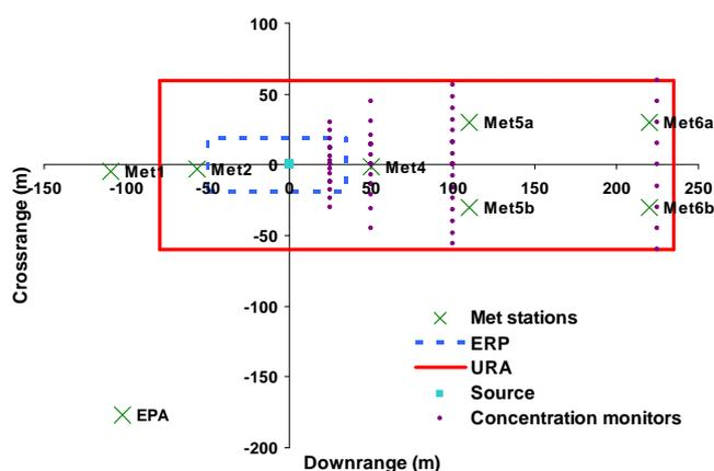
Figure 1. Plot plan of the Kit Fox experiment
