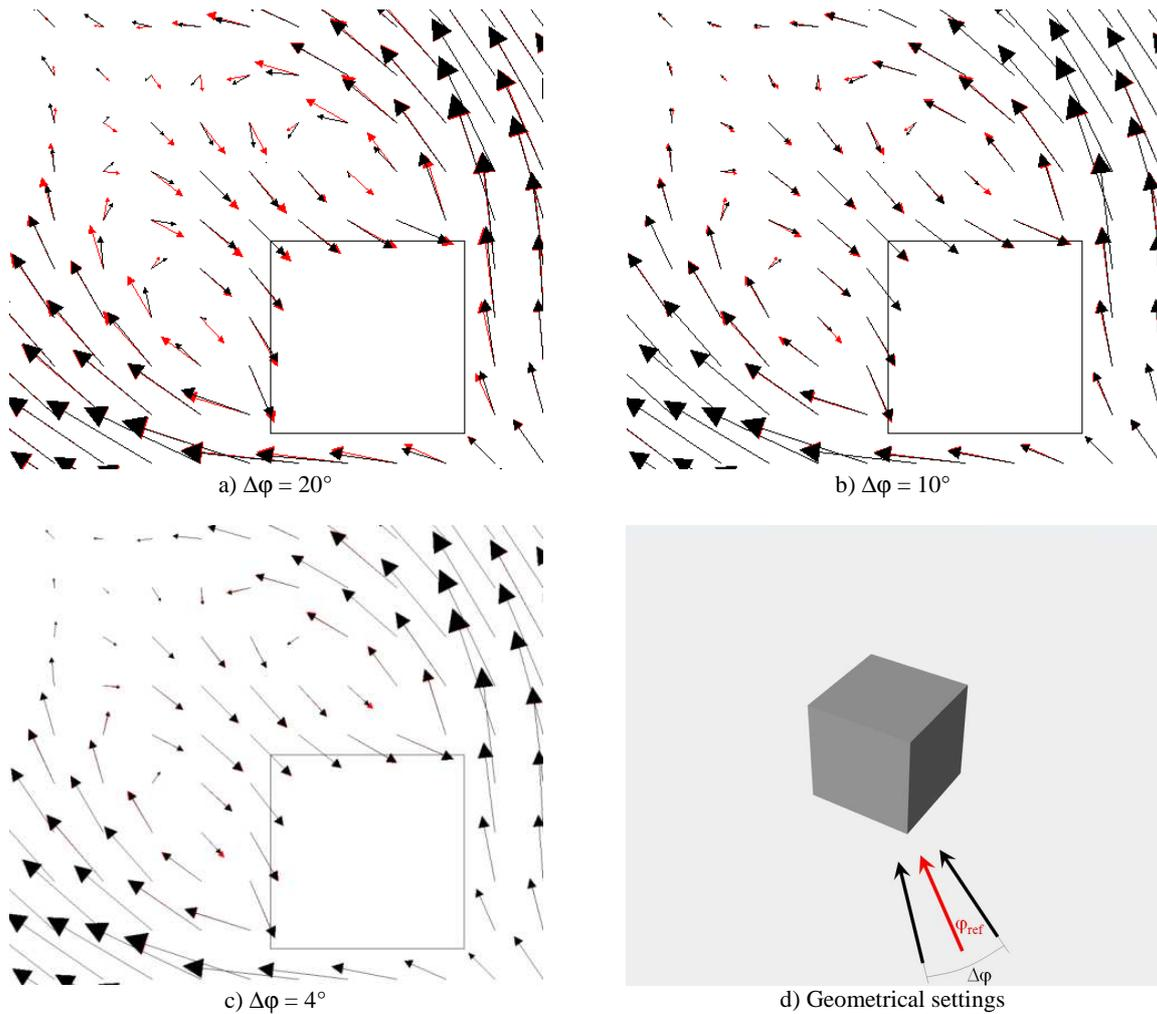
Figure 2. Comparison between the “exact” wind field (in red) and the interpolated wind field (in black) for different interpolation intervals for the wind direction  $\Delta\phi$ .
