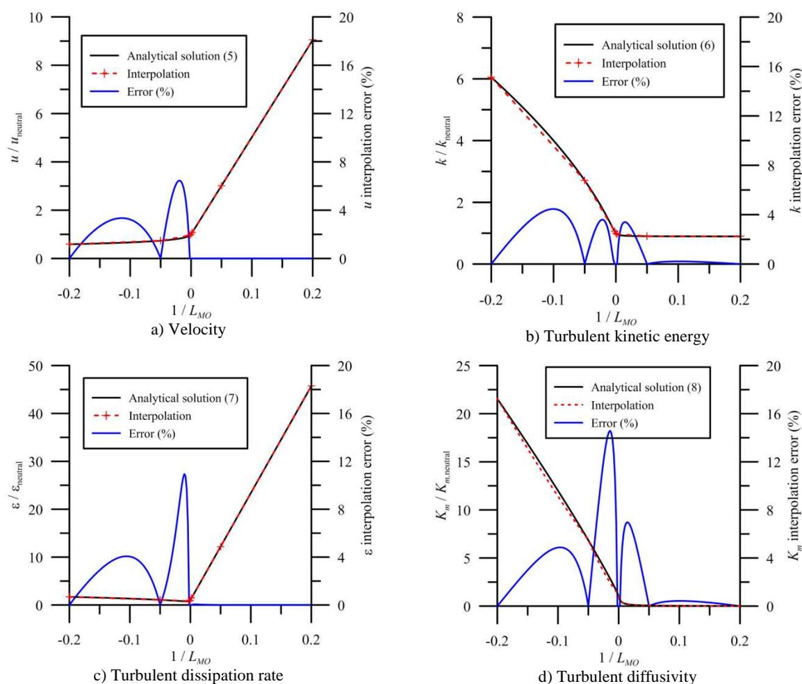
Figure 3. Comparison between the “exact” profiles (in black) and the interpolated profiles (in red) for  $u$ ,  $k$ ,  $\varepsilon$ , and  $K_m$  plotted as a function of the stability parameter  $1/L_{MO}$ . The red cross represents the discrete values of  $1/L_{MO}$ .
