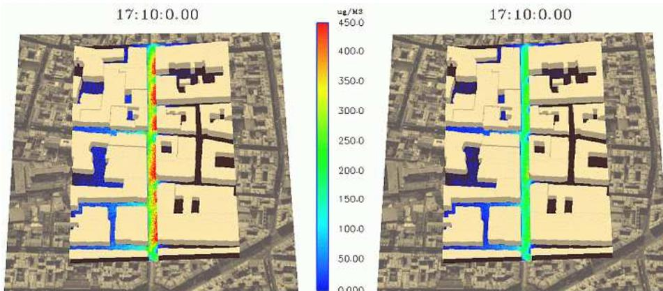
Figure 2: Illustration of the "Street Canyon" geometry (without TiO<sub>2</sub> on the left, with TiO<sub>2</sub> on the right).
