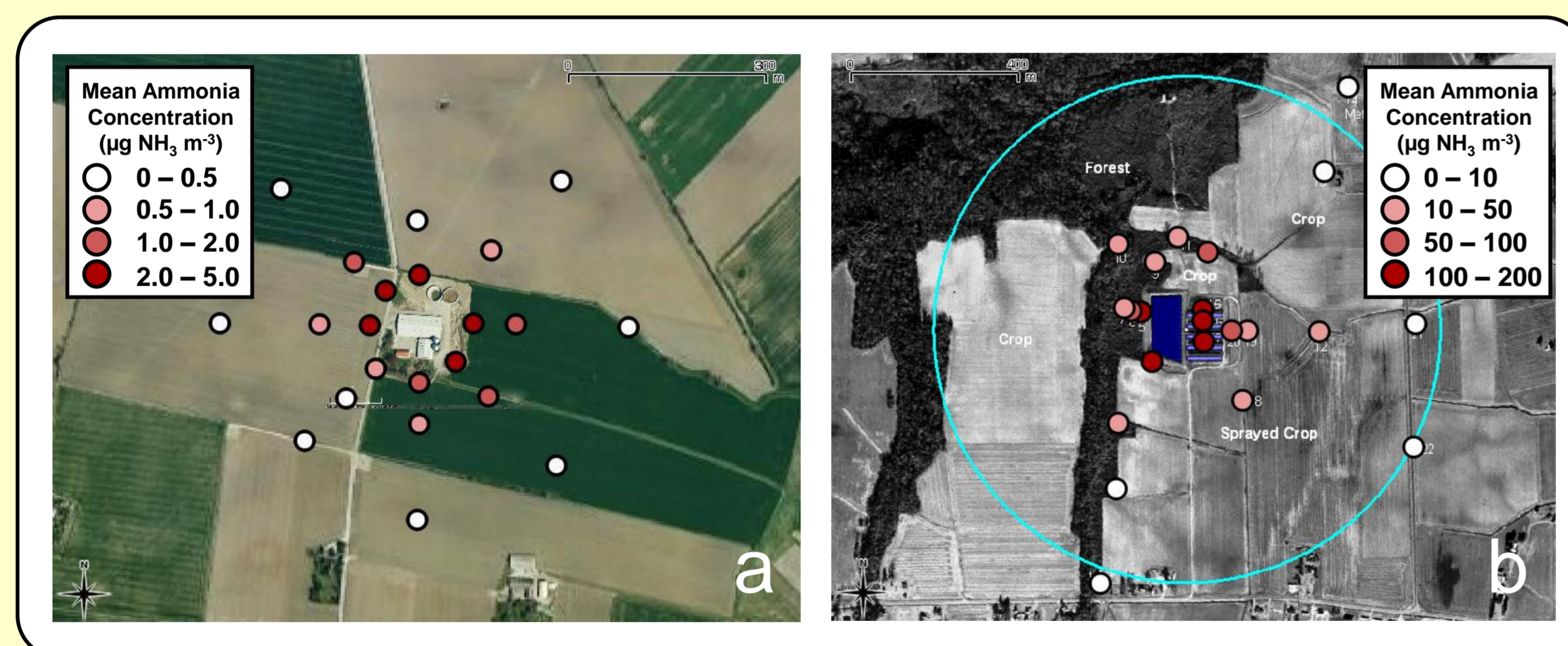
Figure 2a: Mean atmospheric ammonia concentrations measured in the vicinity of a pig farm in Falster, DK 6 .
