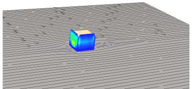
Urban district configuration Streamlines and velocity field at 2 m (The black lines figurate the linear sources of the traffic emissions)
