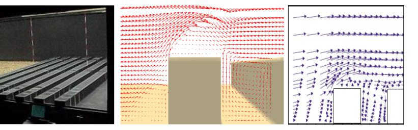
View of the buildings array (left) – Wind field issued by NSWIFT (middle) and measured in a wind tunnel (right) in the vicinity of the first obstacle *N.B. The pressure field is correctly diagnosed by NSWIFT on the front side, but slightly under-estimated at the rear of the obstacle*  • Many validation cases have been carried out in various geometries
