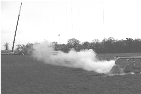
View of a part of the experimental arrangement showing the spill point and vertical steel ropes
