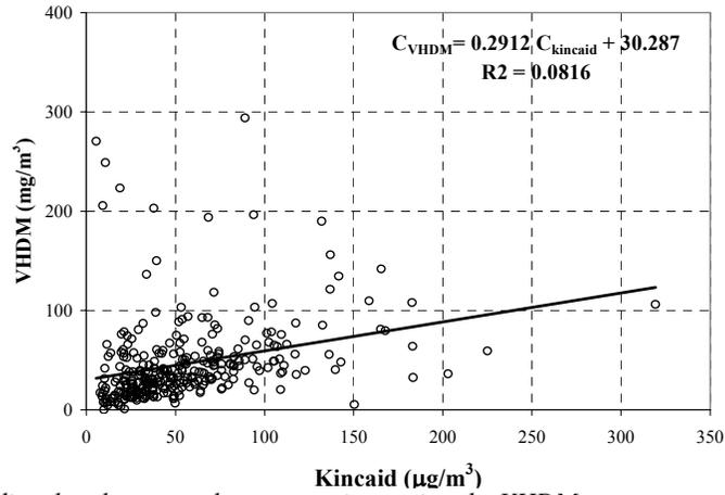
Figure 2. Predicted and measured concentrations using the VHDM.
