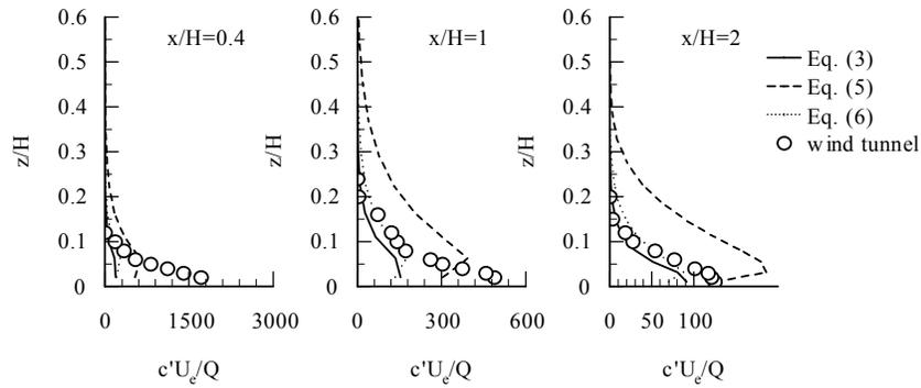
Figure 6. Concentration fluctuations calculated using Eqs. (3) and (6)
