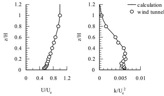
Figure 2. Vertical profiles of mean velocity and turbulent kinetic energy.
