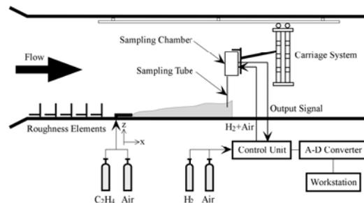
Figure 1. Schematic of the wind tunnel experiment.
