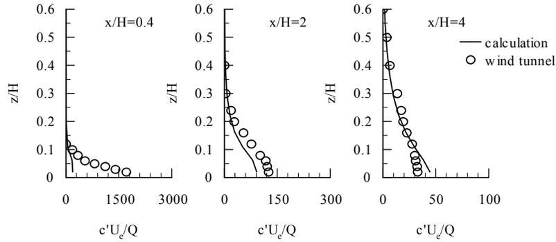
Figure 4. Vertical profiles of standard deviation of concentration fluctuations.
