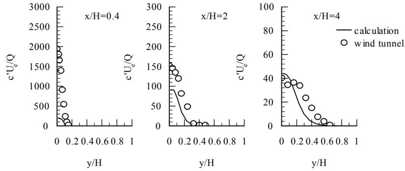
Figure 5. Horizontal profiles of standard deviation of concentration fluctuations.
