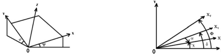
Figure 1. Scheme of the coordinate axes and angles configuration:  $0x, 0x_g, 0x_T, 0x_s$  are correspondingly oriented along the slope, the surface geostrophic wind, the surface thermal wind, the surface wind (North hemisphere)
