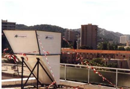
*Picture 1. View of the mini-sodar in the urban station (Marseille, France)*
