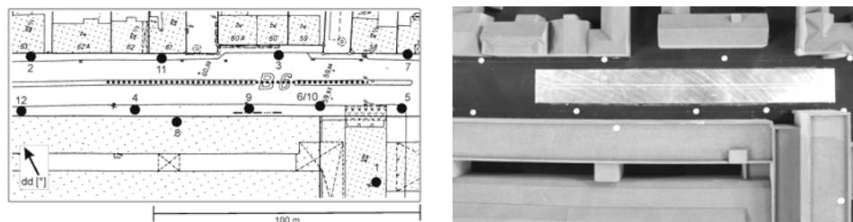
Figure 2. Left side: sampling locations in the street canyon (after Bächlin, 2002), the dotted line represents the line source. Right side: physical model.
